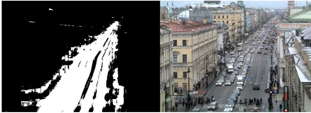
Figure 9 - Road mask generated using accumulated frame difference method(left) and initial image of the road(right)
